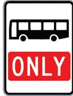
Bus only lane sign
